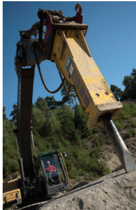
The MB 1650 hydraulic breaker is suitable for carriers between 19 and 32 t
