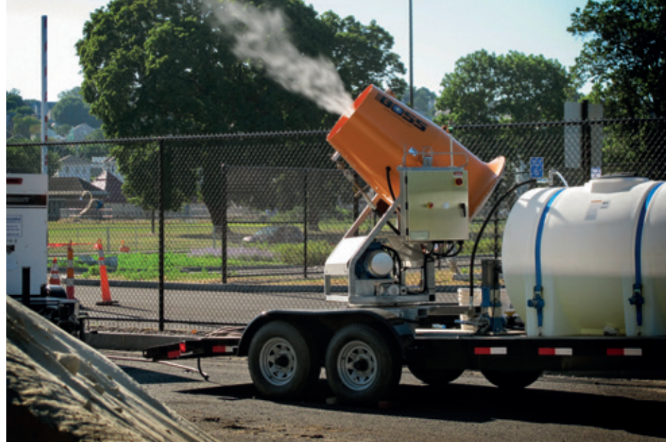
Introducing the mist into an area downwind from the activity allows it to travel with the odour
